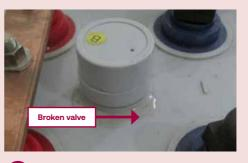
Sign of battery active chemical leakage from the valve.
