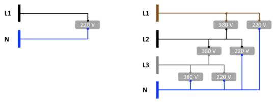
The insulation colours are according to PUIL<sup>1</sup> 2011 and SNI<sup>2</sup> IEC 60445. Previous insulation colours are red for phase 1, yellow for phase 2, blue for phase 3, and black for neutral.
