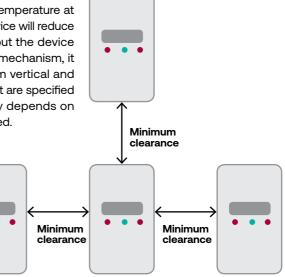
Configuration of SCCs with minimum clearance required by manufacturers. Check the user manual for the minimum clearances.
