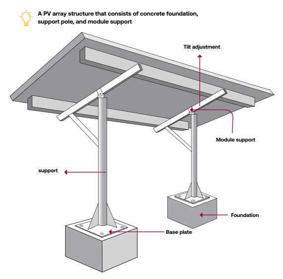
The result of the complete structure should be a sustainable permanent mounting of the PV modules array such as robust and free of corrosion. The array must be installed with correct tilt angle, azimuth<sup>7</sup> angle, sufficient distance between the array and nearby obstacles and with suitable foundation.
