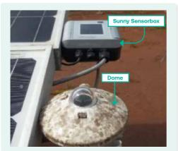
The pyranometer is straightly hit by the sunlight and in the same plane as the PV array. Sunny sensorbox is installed as additional sensor.
