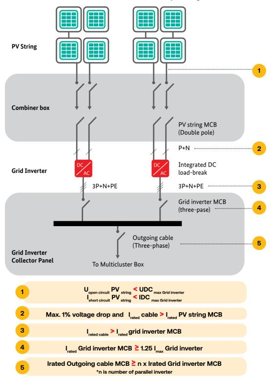
How is the recommended installation when multi-input string inverter is used?
