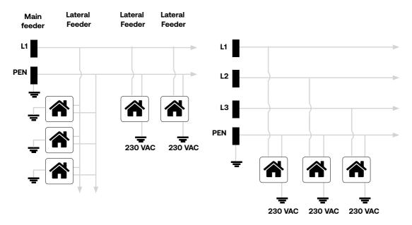
A typical configuration of distribution grid in a village with TN-C earthing system.
