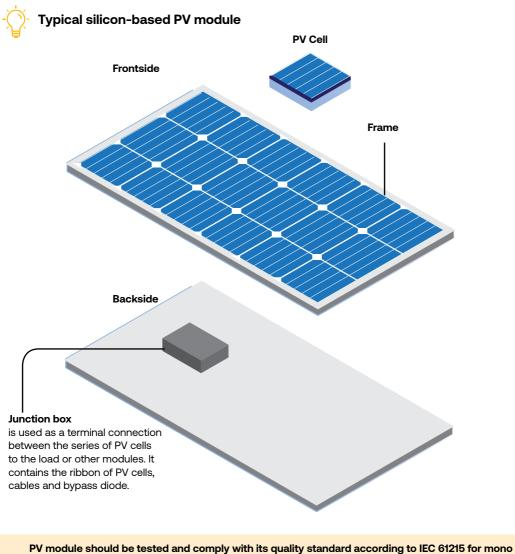
PV module should be tested and comply with its quality standard according to IEC 61215 for mono and polycrystalline module while thin film type adheres to IEC 61646. The modules should also have warranty period that exceeds 20 years operation with maximum performance degradation of 10 % per 10 years.
