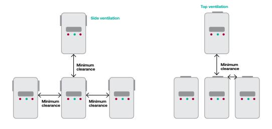
Installation arrangement of battery inverters with minimum clearance for ventilation opening and cable installation. Check the manufacturer instruction for the minimum clearances.
