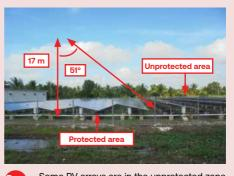
Some PV arrays are in the unprotected zone and at risk for direct lightning strike.
