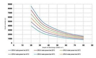
Cycle lifetime of OPzV in the fucntion of DoD and temperature<sup>1</sup>
