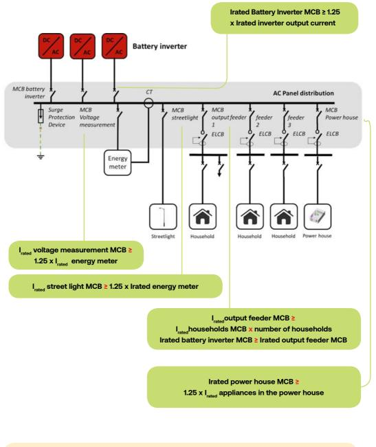
It is recommended that the output feeders should be at least equal to the number of installed battery inverters. This will enable protection coordination which avoid having feeder's MCB (downstream circuit) rating higher than the MCB of the single battery inverter (upstream circuit).
