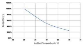
Design life of OPzV as a function of ambient temperature at floating stage<sup>2</sup>
