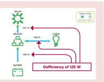
Unrealistic power flow with input power value less than the output. This is caused by one inverter that is disconnected from monitoring device.
