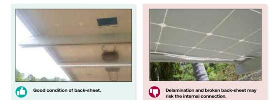
Delamination leads to higher possibility of exposure to live (or electrified) components. The situation might be worsened when the delamination forces the internal connection to break. The broken busbar may create spark gap and thus generate  $\operatorname{arc}^6$  especially at high voltage.
