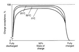
Charge acceptance of sealed lead acid battery<sup>3</sup>
