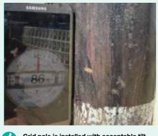
Grid pole is installed with acceptable tilt angle. The tilt angle of the pole should not be greater than 5°
