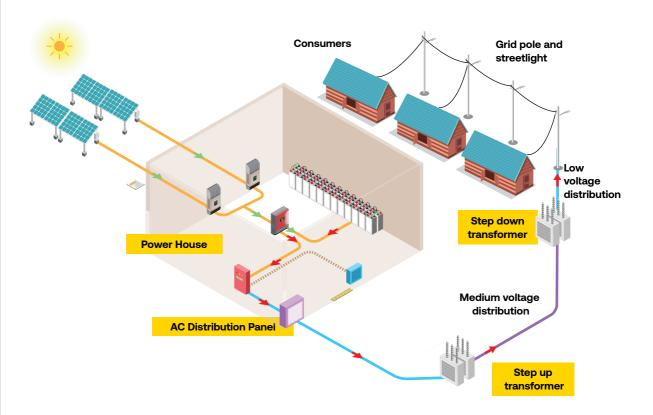
Typical distribution grid in PV mini grid
