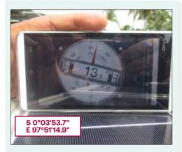
PV modules are located in the equator and are tilted at the angle of 13° to establish self-cleaning mechanism.
