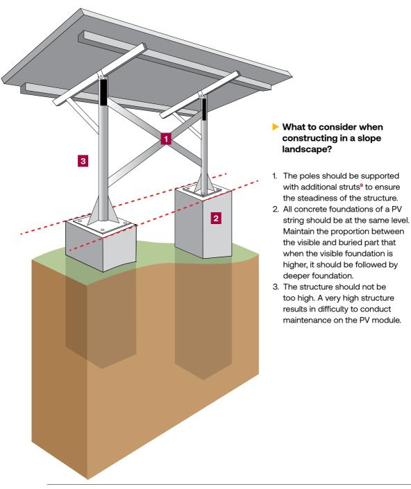
9. Strut is a long, thin piece of wood or metal used for support in a building, vehicle, etc
