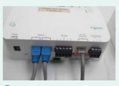
Ethernet cables with strain relief boots are used as cable communication aiming for more robust connection.
