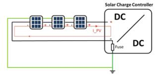
2. Due to some reasons such as corrosion, melting insulation, insulation failures, and bad wiring, short circuit occurs between the exposed positive conductor and the ground. The current path changes and current flows through the grounding cable and internal ground fault protection fuse. The fuse will immediately interrupt the fault and report to the device that ground fault is detected.
