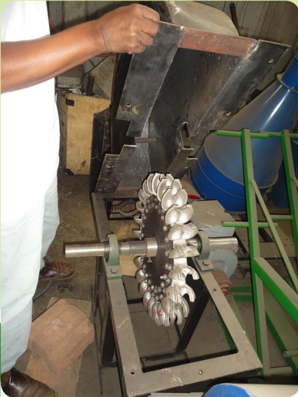
Mozambique: Micro hydro turbine locally produced by Metalurgica in Chimoio, Manica provice
