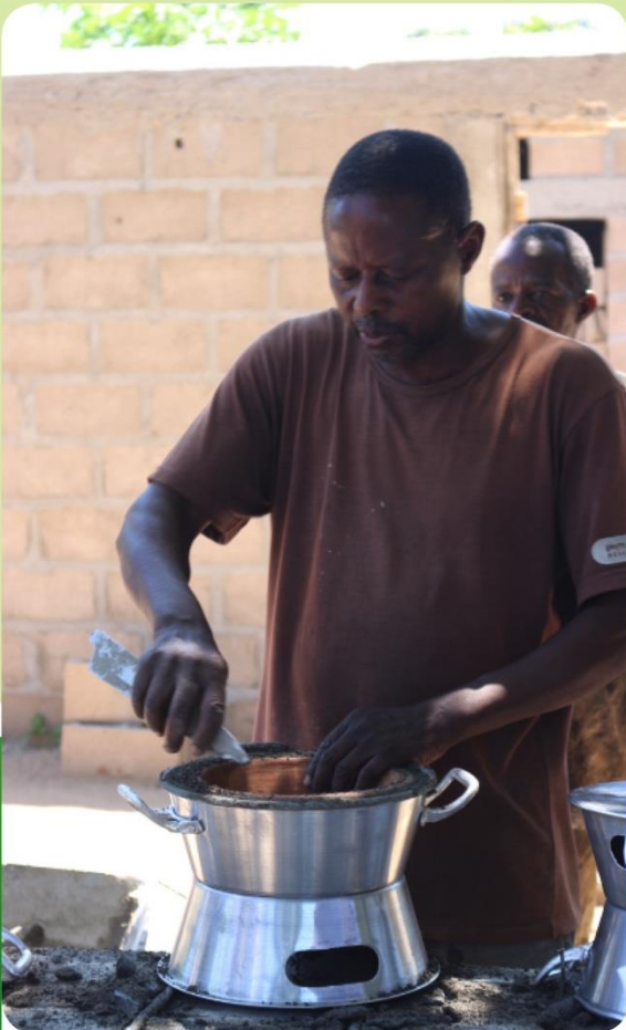
Mozambique: Potter fitting the ceramic combustion chamber in a Mabaula charcoal stove
