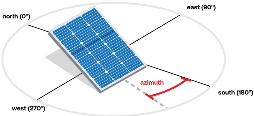
The azimuth angle is also known as the direction where the sun is coming. The PV module should be oriented to face the equator to obtain an optimized energy yield.
