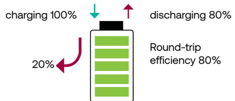
**Round-trip efficiency** is expressed as ratio between the energy used during discharging and energy to restore until its get fully charge. Efficiency includes the losses during discharging and charging. Lead acid battery typically has efficiency of around 85% or slightly lower than lithium ion which is up to 95%.
