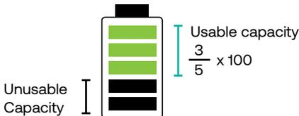
**State of health (SoH)** is the ratio of current condition of battery to the ideal or the capacity when it is new. It is expressed in percentage %. One of the reasons of the reduction of SoH is due to increase of internal resistance of the battery that makes some part of battery capacity unusable
