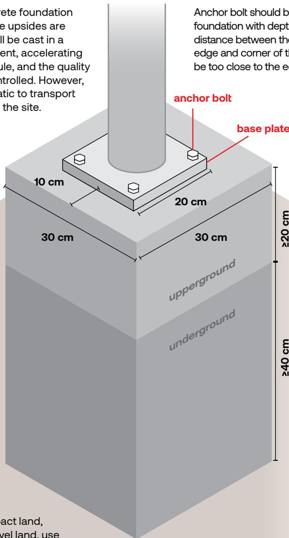
Construction of foundation should comply with a minimum dimension of 35 cm x 35 cm x 60 cm (length x width x height). If 60 cm of height is used, the installation depth of the foundation should be at least 40 cm or two third of total height (20 cm remains visible).
