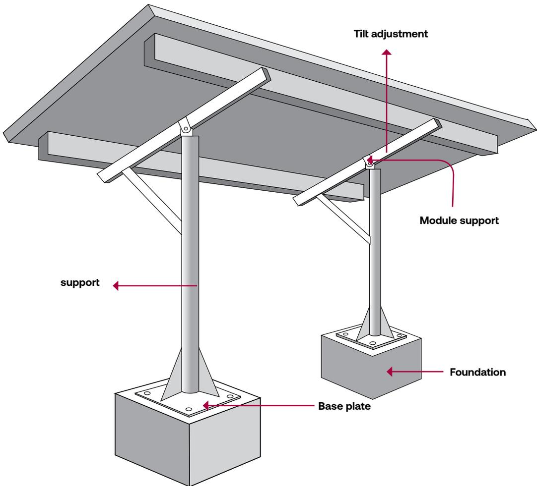
The result of the complete structure should be a sustainable permanent mounting of the PV modules array such as robust and free of corrosion. The array must be installed with correct tilt angle, azimuth<sup>7</sup> angle, sufficient distance between the array and nearby obstacles and with suitable foundation.
