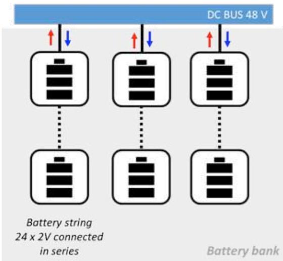
Typical installation of the lead-acid battery bank inside the power house. Battery bank is configured from several battery cells connected to series or parallel to achieve the intended system voltage and capacity.
