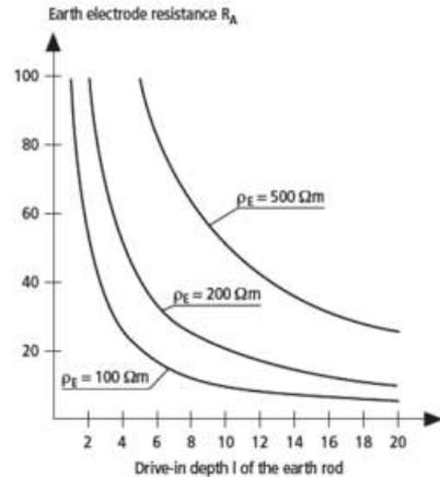
**Resistance ( $R_A$ ) of grounding electrode vs its length<sup>2</sup>**
