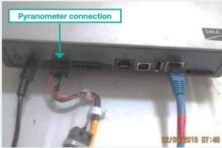
**Pyranometer is connected to monitoring device via RS485 interface**
