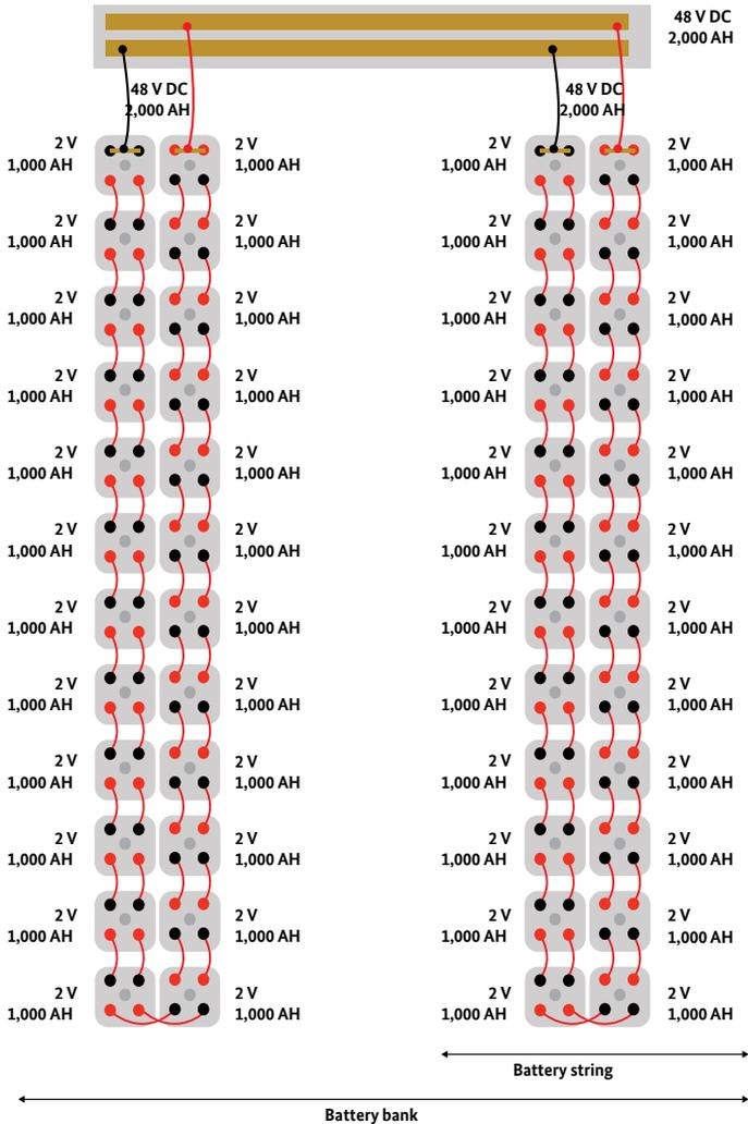
► **What should be considered when connecting the batteries?**
