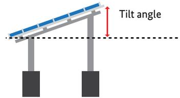
The tilt angle can be measured using clinometer or protractor.
