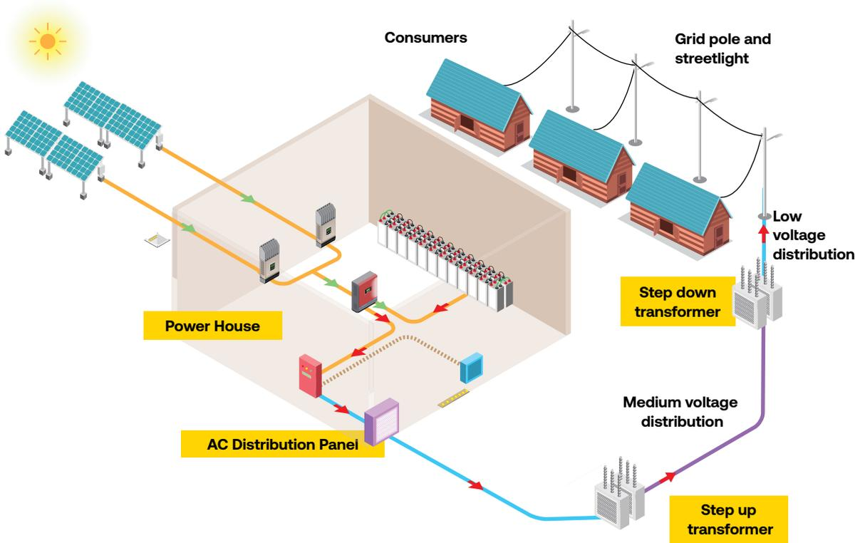
Typical distribution grid in PV mini grid
