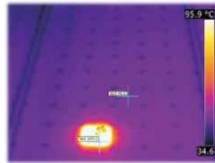
Detection of hot spot on a PV module. There is a block of cell that has significantly higher temperature compared to the neighbouring cells.
