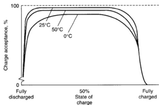
Charge acceptance of sealed lead acid battery<sup>3</sup>
