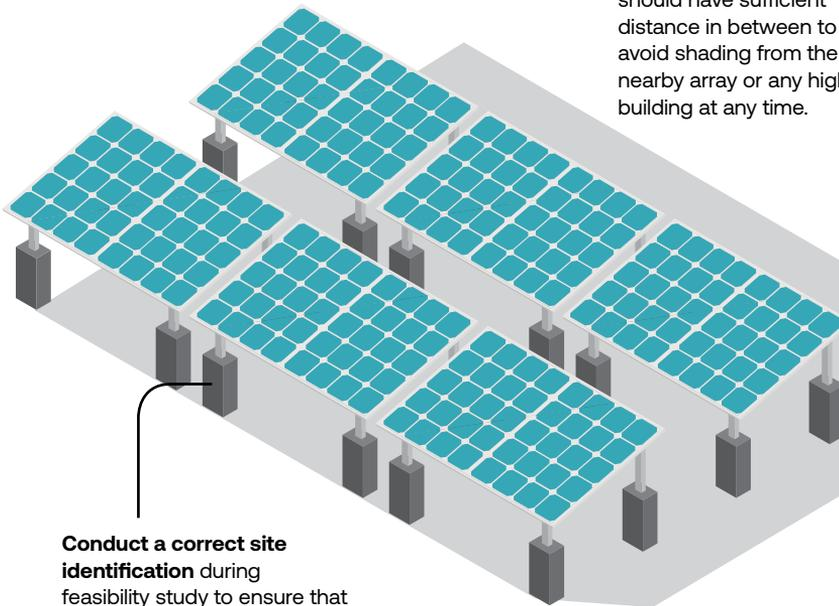
📄 **Verify during commissioning process whether the PV arrays are clear from shading** at any time and consider the potential shading in the future such as growing tree.
