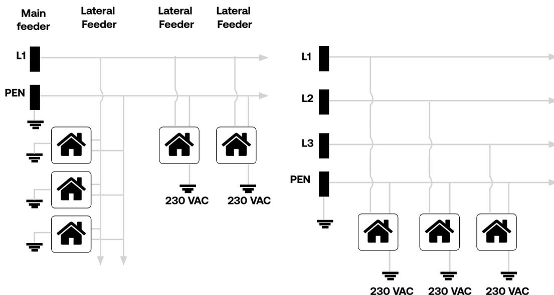
A typical configuration of distribution grid in a village with TN-C earthing system.
