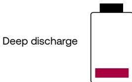
**Deep discharge** is when the battery is discharged below the end-of-discharge voltage. End-of-discharge voltage itself is the voltage point of the battery when the battery has completely discharged or when its SoC is less than 20%
