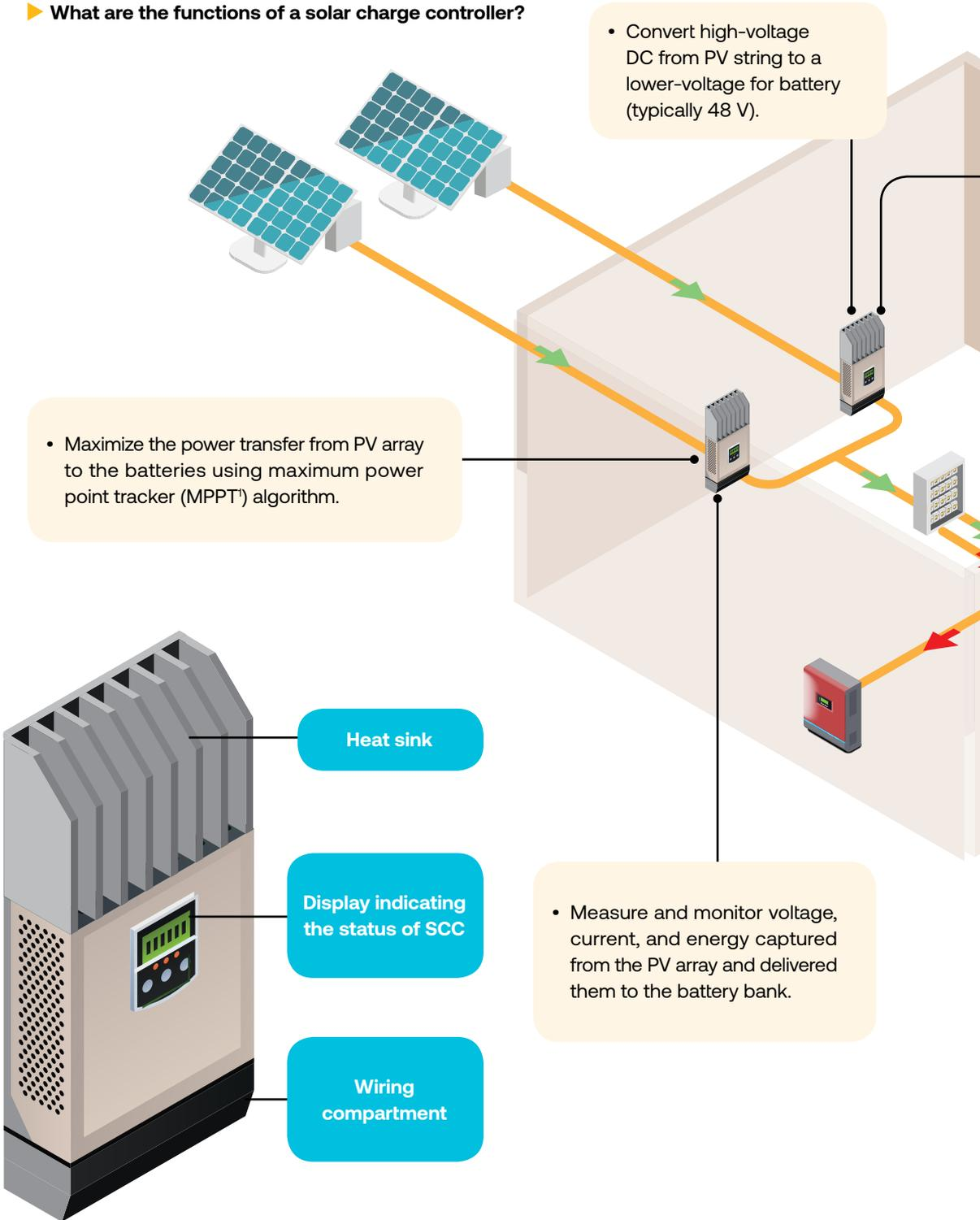
1 Maximum Power Point Tracker is an algorithm or technique used by solar charge controller or grid inverter for tracking and extracting maximum possible power from PV array under certain conditions.
