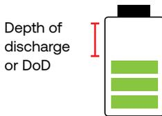
**Depth of discharge or DoD** is the amount of energy used from the battery. It is the opposite of state of charge. Therefore, when a battery specifies its lifecycle might be greater than 1500 cycles with 80% DoD, meaning it will only occur if the usage of energy is not higher than 80% of the nominal capacity.
