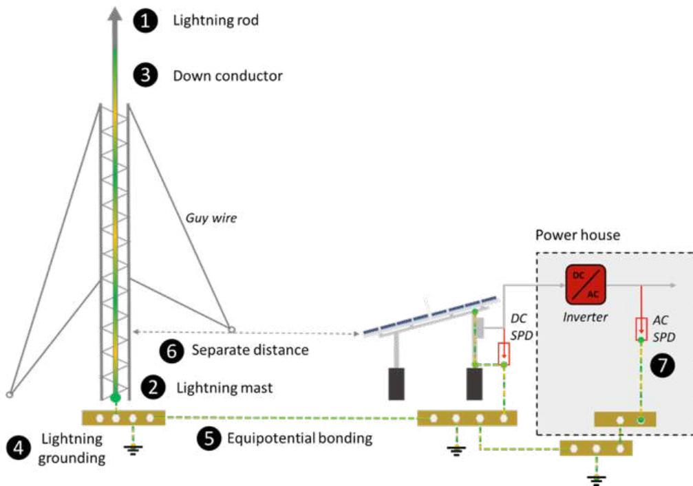
1. **Lightning rod** provides path to ground that can be used to conduct the high lightning currents when lightning strikes occur or to intercept the lightning flash.
