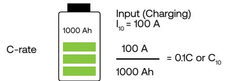
**C-rate** is typically expressed as the charge or discharge rate equal to the battery capacity divided by time. For example: a C10 discharging rate (or I10 for 1000 Ah would be 1000/10 or at 100 A.
