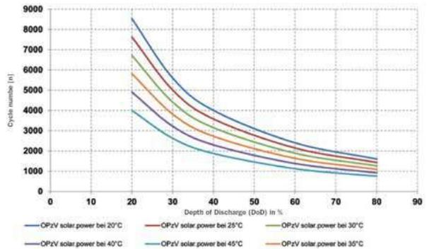
Cycle lifetime of OPzV in the function of DoD and temperature<sup>1</sup>
