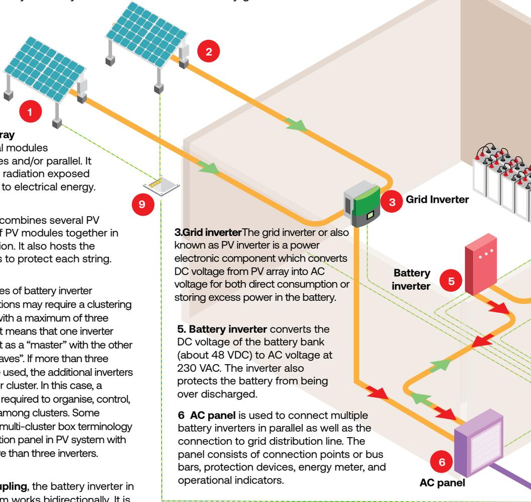
**1. Photovoltaic array** consists of several modules connected in series and/or parallel. It converts the solar radiation exposed to the entire array to electrical energy.
