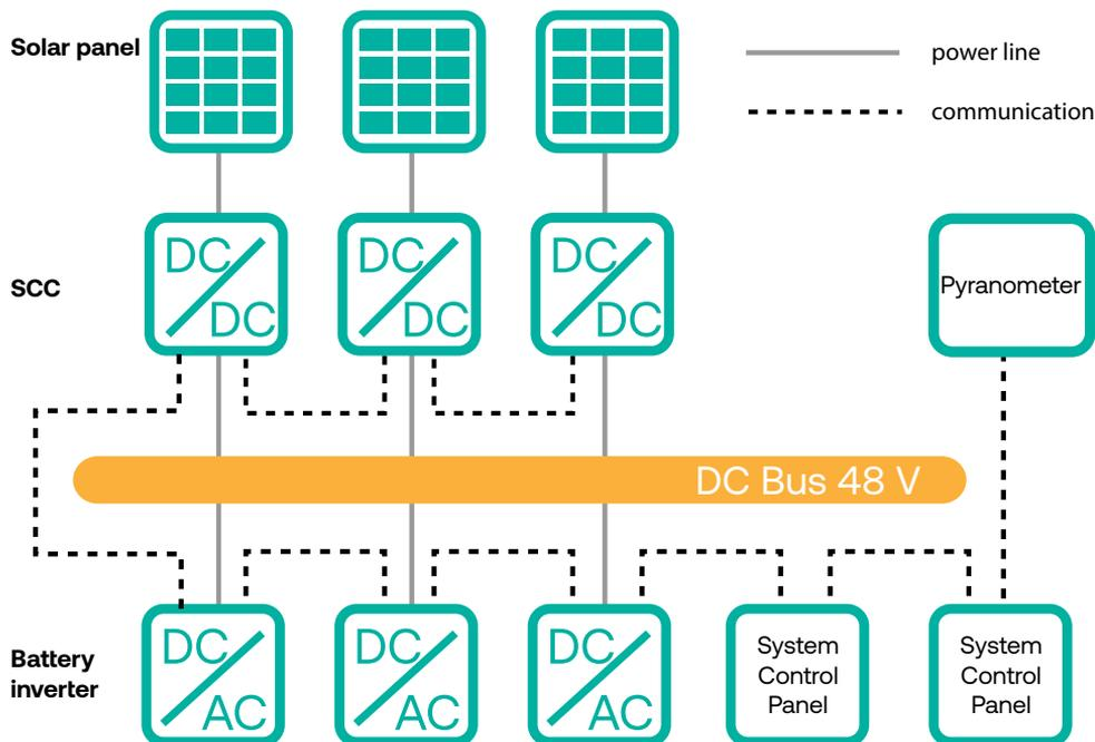
**Typical installation of the monitoring system. Cable communication is connected in daisy chain<sup>1</sup>.**
