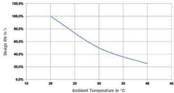
Design life of OPzV as a function of ambient temperature at floating stage<sup>2</sup>
