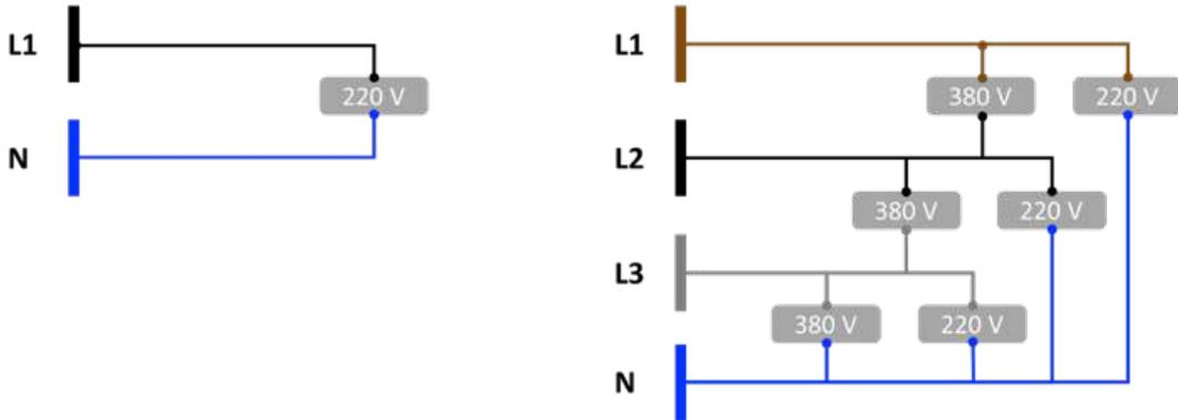
The insulation colours are according to PUIL<sup>1</sup> 2011 and SNI<sup>2</sup> IEC 60445. Previous insulation colours are red for phase 1, yellow for phase 2, blue for phase 3, and black for neutral.
