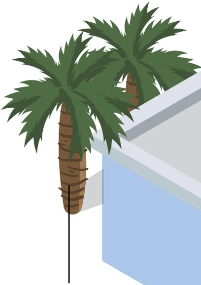
✂ **Vegetation under and surrounding the PV arrays should remain low.** It is necessary to conduct vegetation clearance during periodic maintenance.
