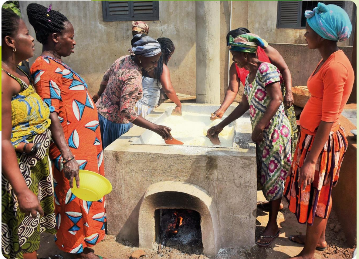
Ghana: ICS for gari roasting in the Tsormenyo Gari Processing Centre, Mafi Kumase Community, Volta Region. EnDev cooperates with SNV in Ghana to introduce improved Gari roasting stoves for SME so that agro-processing industries become familiar with the financial and health benefits of improved cookstoves.
