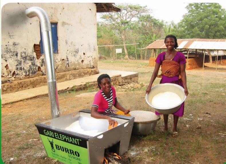
Ghana: SNV conducted a study, according to which an ICS for Gari processing can reduce fuelwood consumption by 30%, and hence induce cost savings. SNV estimated a market potential for up to 50,000 improved institutional Gari cookstoves. The new option is the burro, Gari Elephant. It is expected to augment the net income by at least 20% and a payback time of under 6 months.
