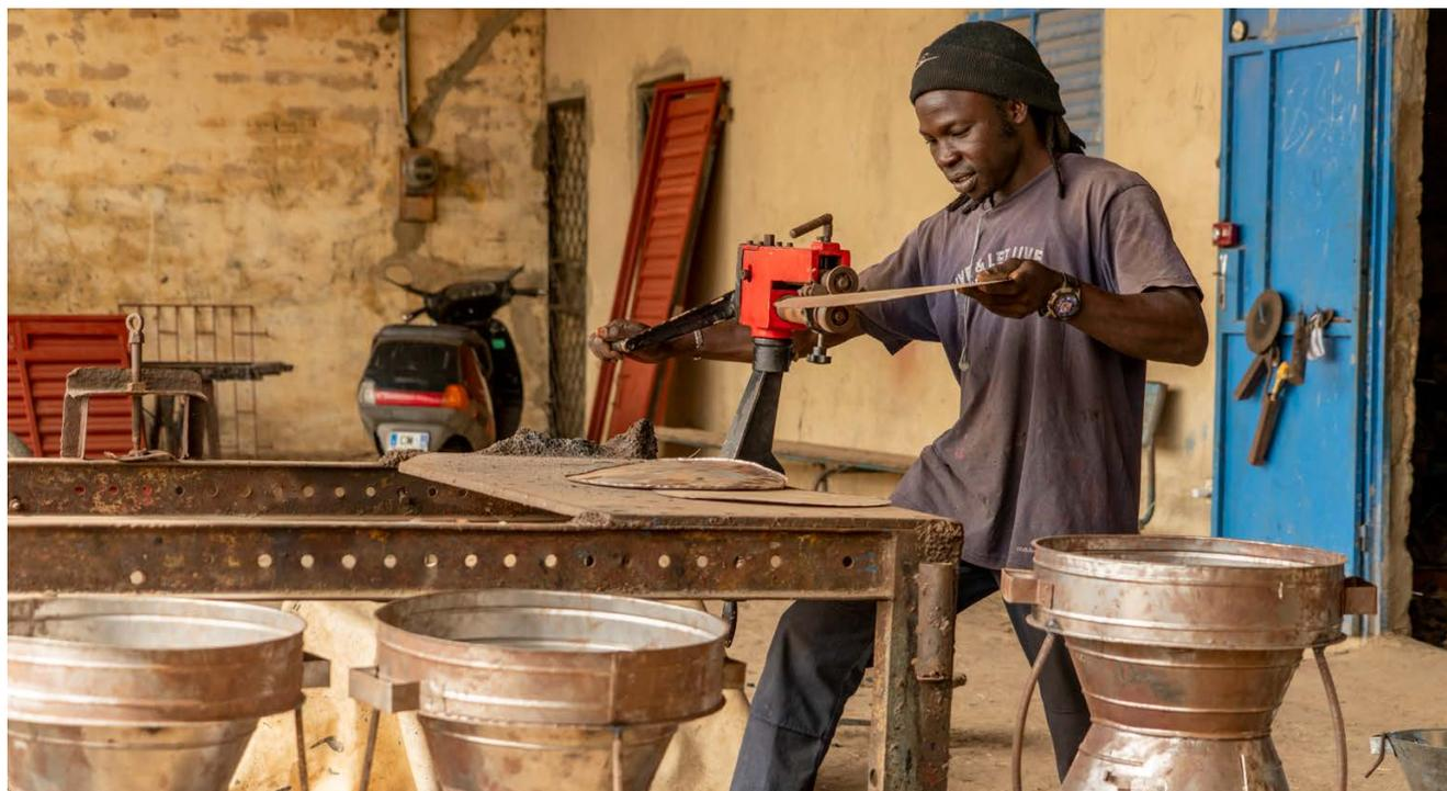
Modou Gamou is bending the metal for the metal cladding of the main body of the ICS in Sokone Kaolack, Senegal
