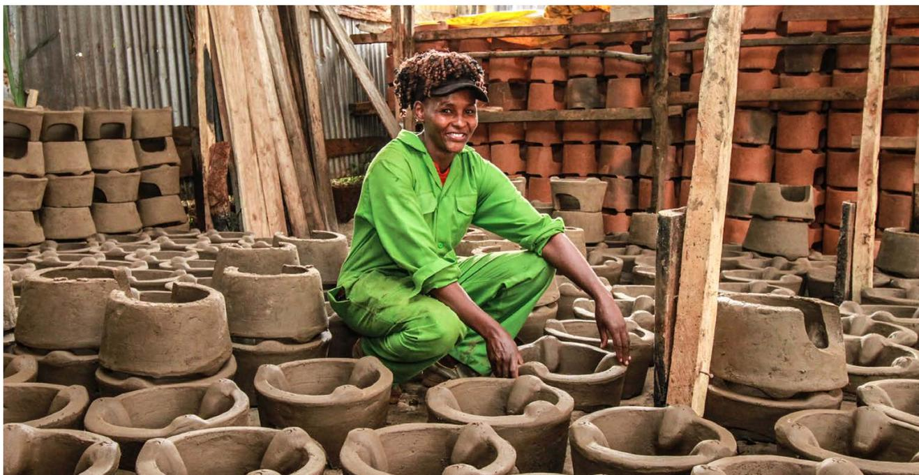
Naomi Ngotho the owner of Naomi production center is stacking the ceramic parts of the ICS for drying. The workshop is located in Muranga, Kenya.
