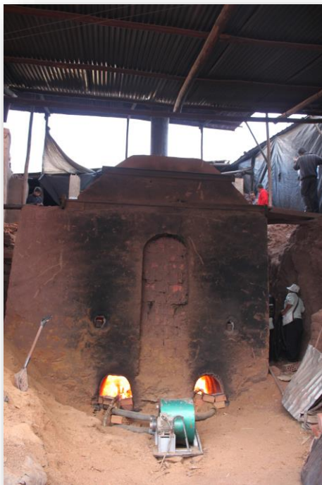
An improved brick oven, one of the productive use technologies promoted under the competitive grant component of FASERT
