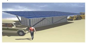
Figure 1: General design of a solar container (source: GIZ)
