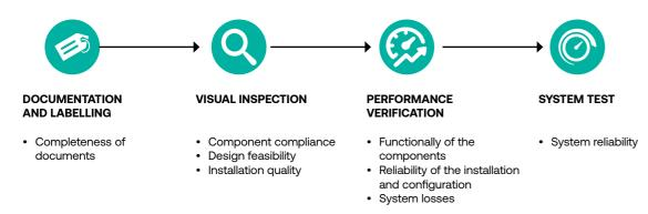
data will be recorded by a data logger and system performance during this commissioning period will be analysed. Below figure illustrates the steps and activities for PV mini grid commissioning. The duration of implementation can vary depending on the weather conditions during commissioning activities.
