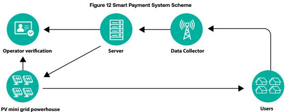
The SPS is designed to automate energy management in a such way that excess energy can be used by households who have subscribed to utilise the excess energy. It has an algorithm that provided several options for daily energy limit in each household, which enables several households to consume excess energy that is available during daytime.
